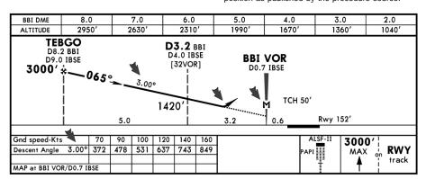
In exceptional cases it may be necessary to include both, CDFA and non-CDFA/other than CDFA flight path. In this case, a level segment is shown prior to the missed approach point and the pull-up arrow is shown at the MAP to depict the non-CDFA/other than CDFA procedure.
